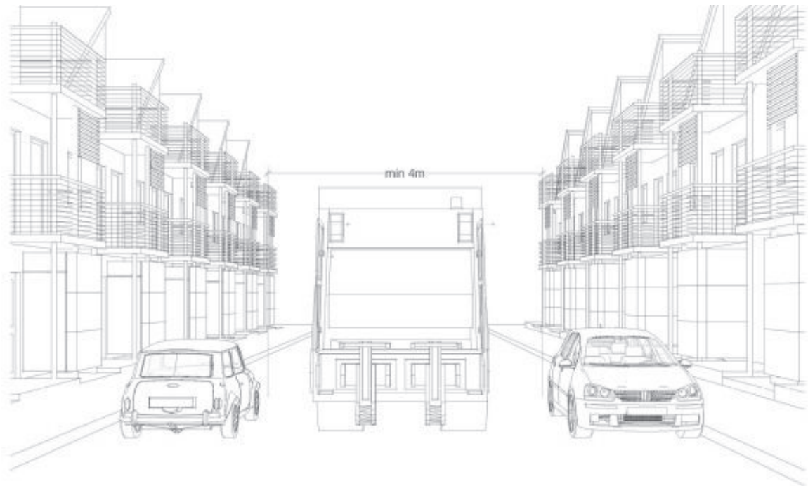
Diagram 6.3 - An example of minimum road width clearance required where on-street parking is provided for on both sides of the road
