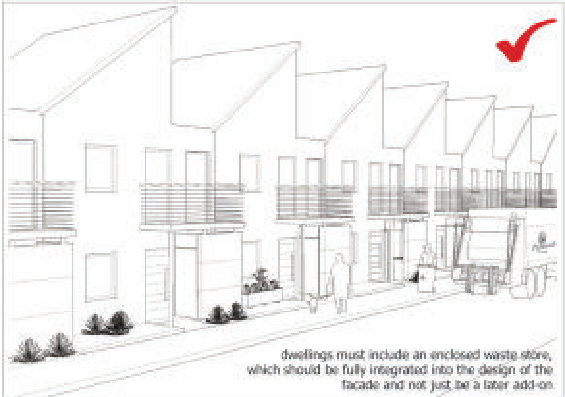
Diagram 6.2 - Good and poor examples of provision for bin storage in residential design
